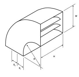
\*All fittings are available with acoustic lining or double wall construction.
