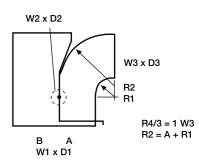
Splitter Damper Length is Equal to 1.5 A Where: A = 100 mm Min.
