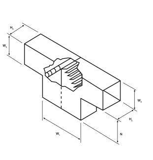
\*All fittings are available with acoustic lining or double wall construction.
