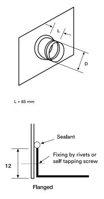
\*Application of sealant after installation is recommended. \*For "D" dimensions, please see the Flexible Duct catalogue or the Round Duct and Fittings catalogue for spiral duct dimensions.
