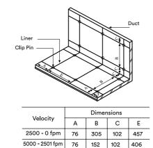
Liner bonded to duct with adhesive and welding pins at approximate centers as shown.
