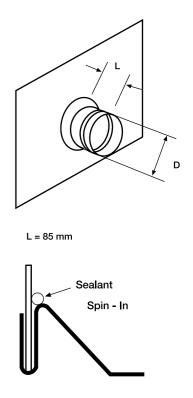
\*Application of sealant after installation is recommended. \*For 'D' dimensions, please see the Flexible Duct catalogue or the Round Duct and Fittings catalogue for spiral duct dimensions. \*All fittings are available with acoustic lining
