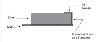
Liner to be 48 kg/m3 (3 lbs/ft3) density, 25 mm thick, unless otherwise specified.
